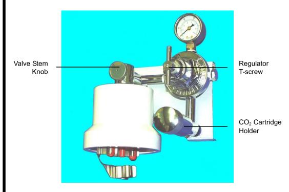
3. Remove the CO<sub>2</sub> cartridge holder and insert a new cartridge. Turn the regulator T-screw completely counter-clockwise. Puncture the CO<sub>2</sub> cartridge by tightening the holder.
